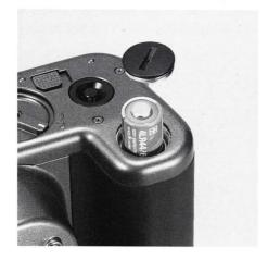
Insert the battery as shown in the Photo, being sure to properly place the battery with the "+" side up, facing the cover.
