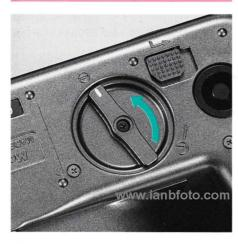
Rotate the light shield closing lever in the direction of the arrow, away from the open position "  $\supset$ " and align the white indicator on the lever with "  $\rightleftharpoons$ " to close.
