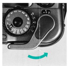
Wind the film advance lever until it stops automatically and "1" appears in the exposure counter window.
