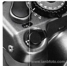
When it is lightly touched, correct metering data is displayed on the bottom of the view finder. When it is depressed all the way, the shutter is released.
