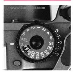
Rotate the shutter speed dial and select either the A (Auto exposure) or manual mode for photographing. Set the film speed of the film being used by lifting up the outer rim of the shutter speed dial and rotate it until the correct ISO value appears in the window.
