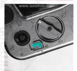
Slide the light shield curtain release lever along to follow the arrow"
