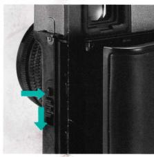
While depressing the back cover lock release button, simultaneously push down the back cover latch in the direction of the arrow.
