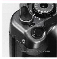
(ON) Align the white dot on the lever with the white dot on the camera body.
